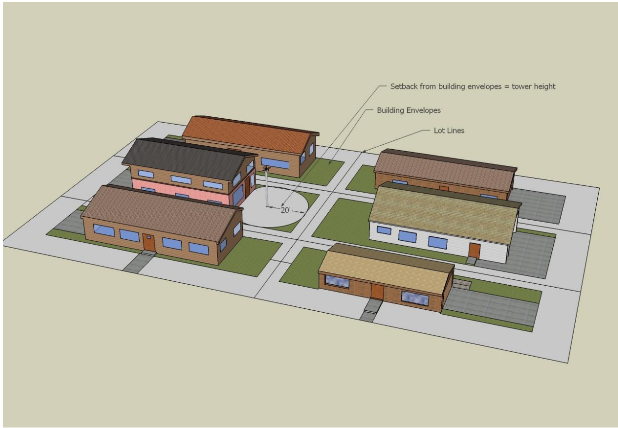
FIGURE 9 SMALL WIND TURBINE CLEARANCES
